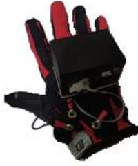
Figure 1- HMI (glove) Prototype
